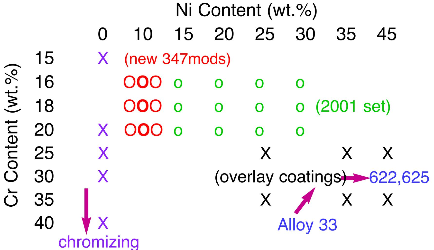
Cast 400g, hot-roll to 8mm: cut coupons & rods
