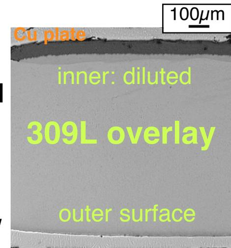
Rectangular coupons: removed overlay from tube
