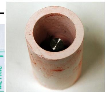
25x6mm rod in porous alumina
