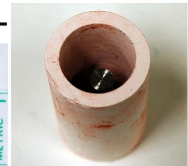
25x6mm rod in porous alumina
