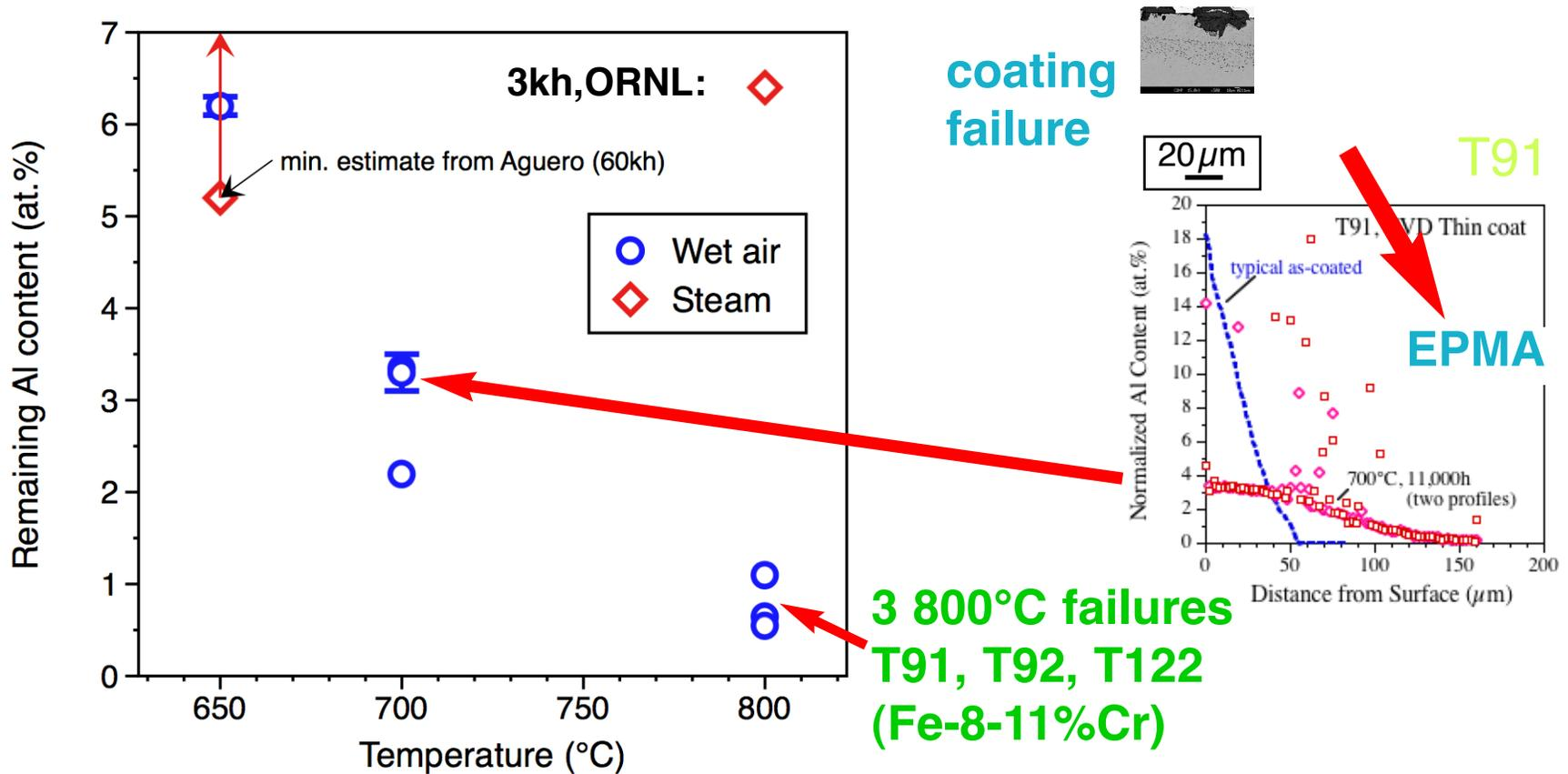
Six failures of thin coatings, one higher Al activity coating
