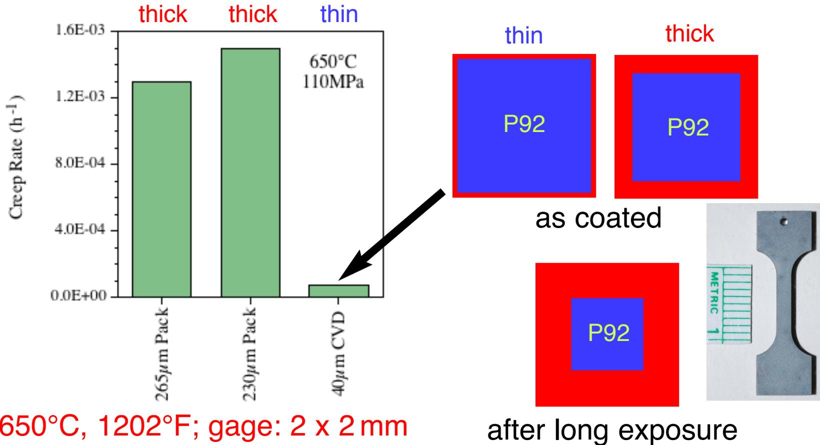
Specimen with thin coating has better creep resistance
